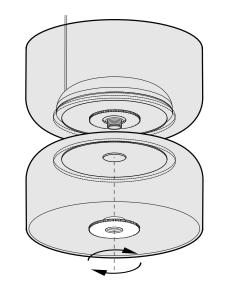
**4** Thread the LED MODULE onto the lamp assembly.
